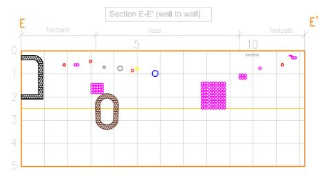
Ground Penetrating Radar survey (plan top and section below) of services and utilities underneath a city centre street.
