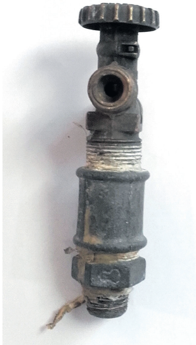
Photograph 5: Turn down valve i.e. screw on H valve.
