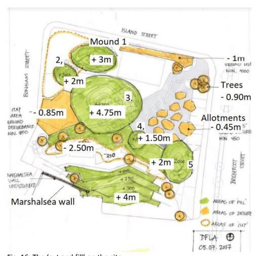
Fig. 16: The 'cut and fill' on the site
