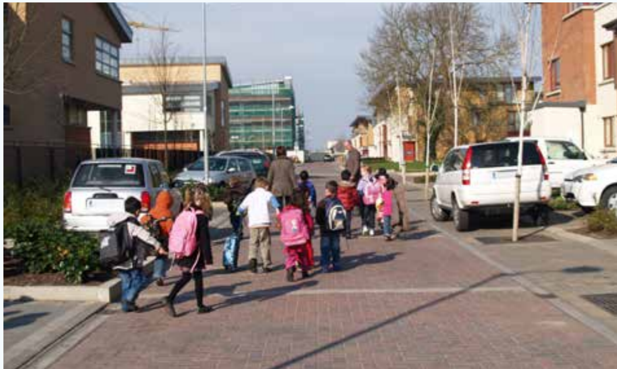
Traffic calmed home zone style street with changes in materiality to demark parking bays and verges.
