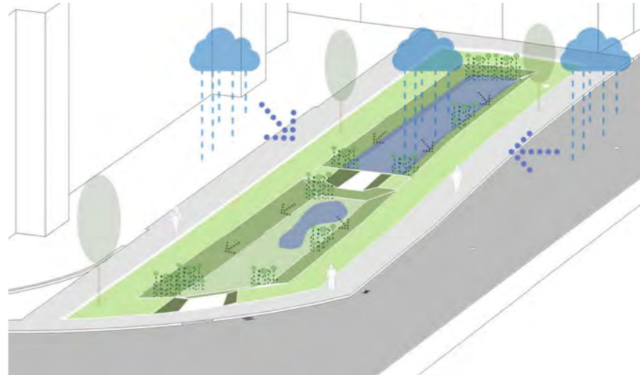
02 - Surface water run-off from roads, footpaths and buildings is directed and channelled to the green space where it begins to accumulate in the hollows.
