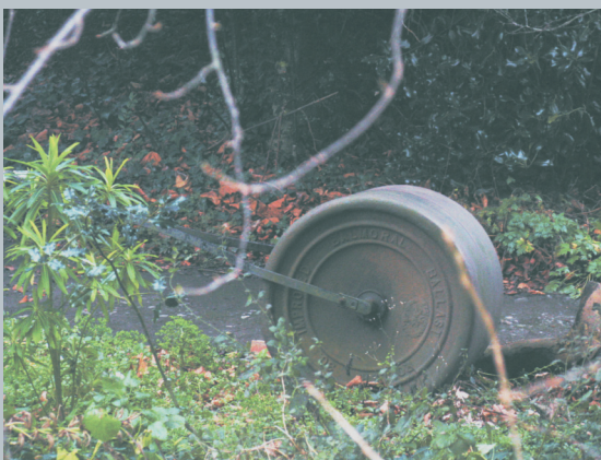
Photo 2.1.6.5 Ballast lawn roller
