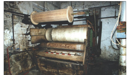
Scouring dolly, Building 1A
