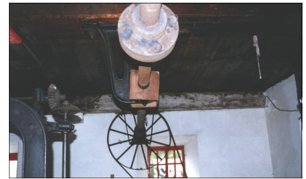
Transmission shaft fixed to underside of floor
