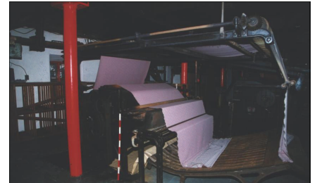
Steam brushing machine, Building 1
