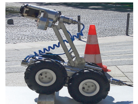
CCTV Camera with elevator
