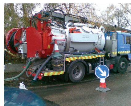
One of DCC's high pressure jetting and vacuuming machines
