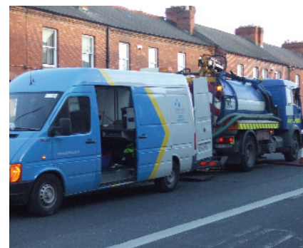
CCTV Van and High Pressure Jet Vector
