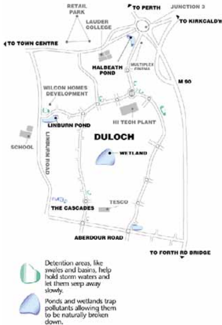
Figure D1 Layout of SUDS at the DEX Site
