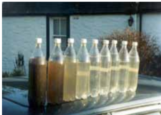
Visual evidence of improved water quality along the Briery Hills Treatment Train.
