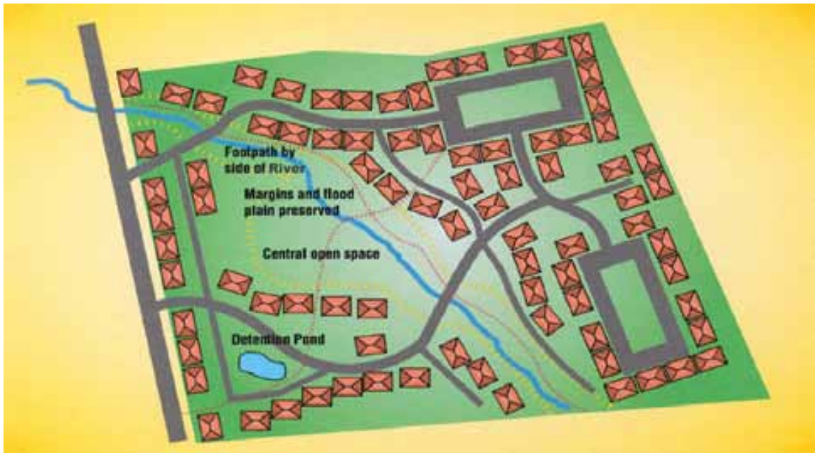
Figure 30: Plan of Development centred on river frontage, incorporating flood plain and SuDS facilities
