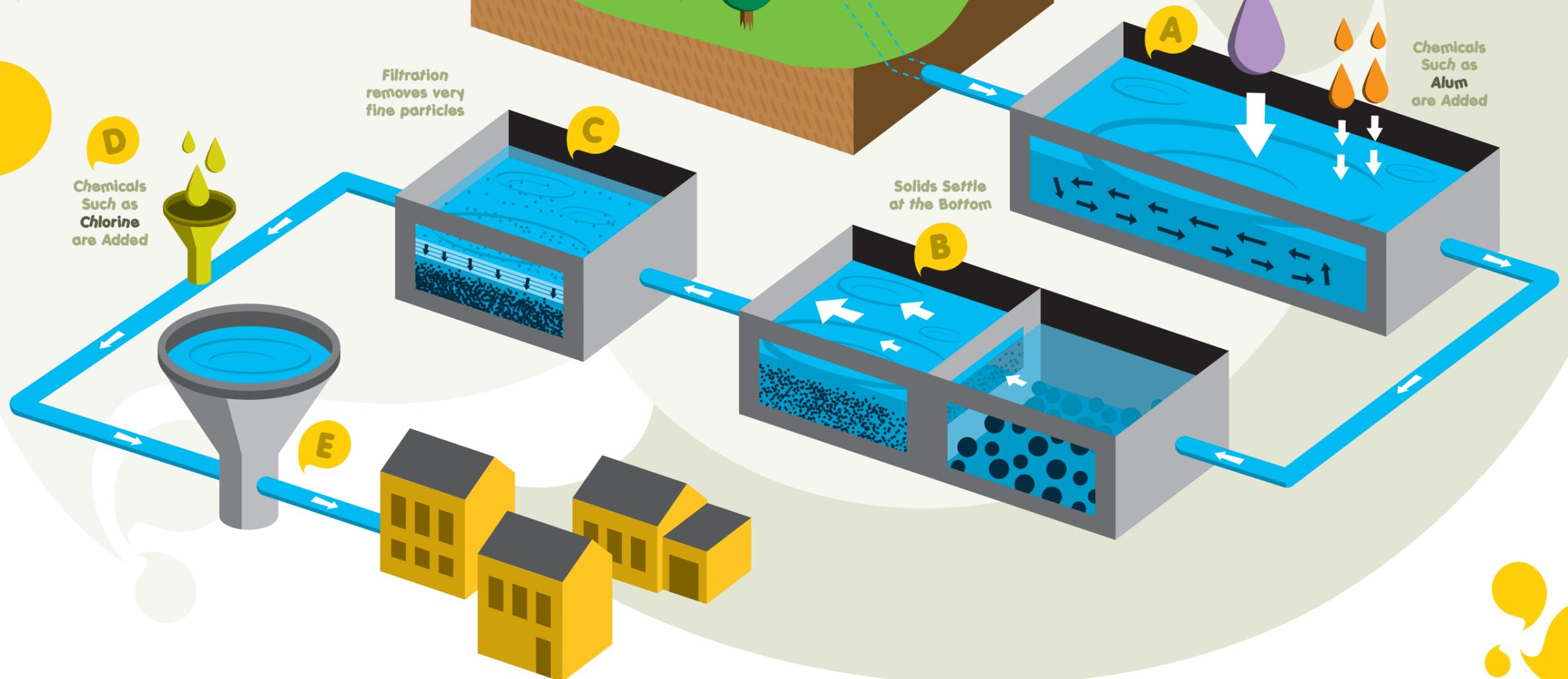
**C** The clear water at the top is then passed through filters, which are made of sand and gravel, and remove any remaining 'suspended matter'. This is known as **filtration**.
