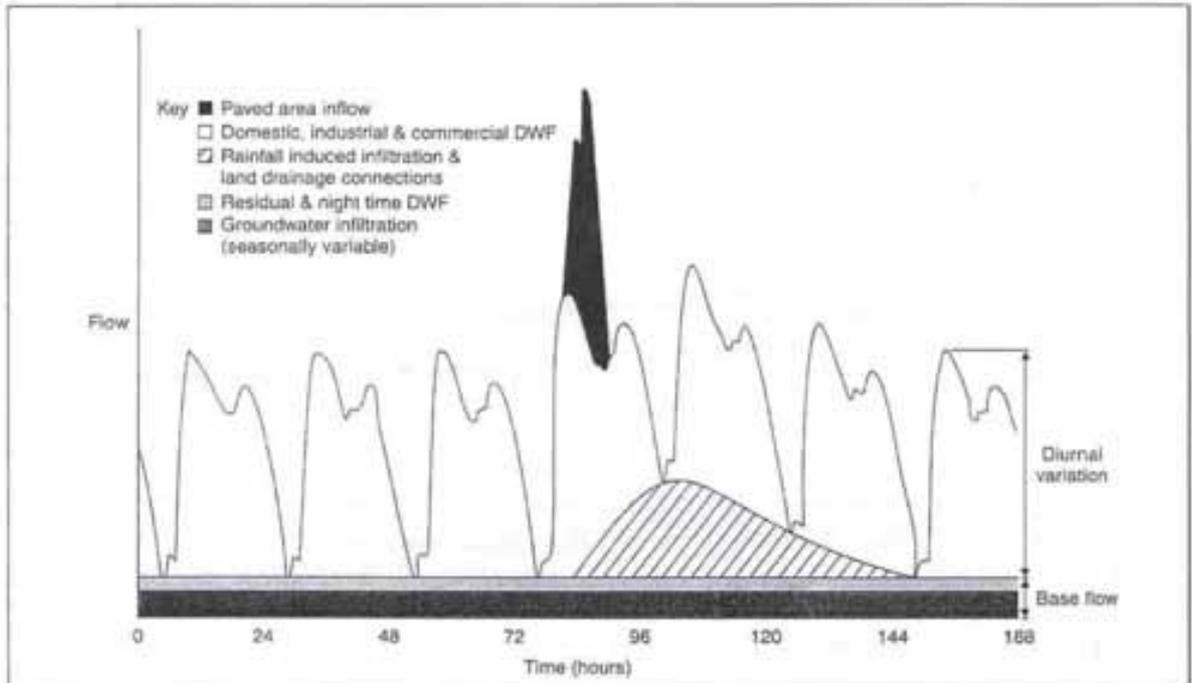
**Figure 2.1 The Components of Flow in a Foul/Combined Sewer System**
