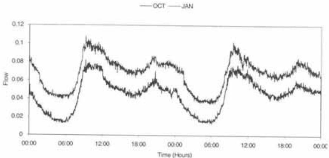
**Figure 2.4 Seasonal Variation in Infiltration** (Dry weather flow in sewers (CIRIA 1998))
