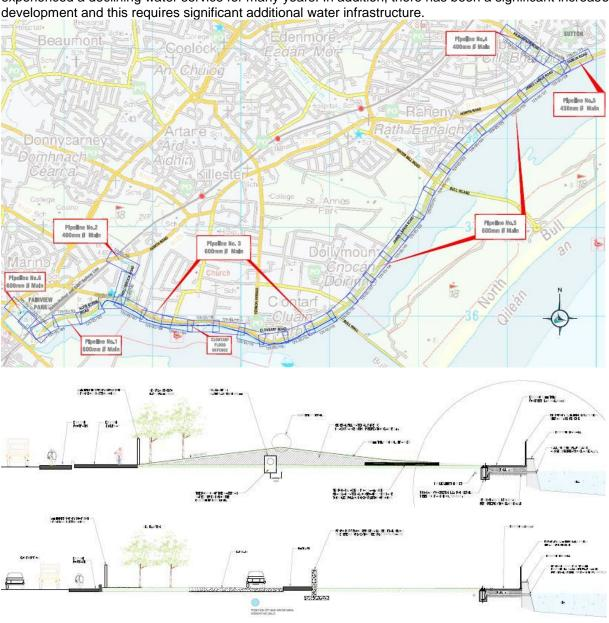
The North Fringe Water Supply Scheme involves the construction of 36km of watermains from Cappagh Cross to Baldoyle and a major ground level reservoir and high-level water tower at Sillogue. The scheme will also create a new trunk 'Ring Main' connecting the network from different sources. This scheme will improve the water supply and water pressure in the North City and South Fingal areas.
