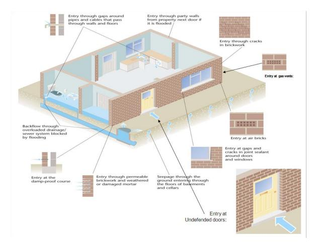
Doors, low windows, air bricks, broken brickwork, backflow of sewerage up through the toilet and ground water pushing up under the floor, are just a few of the many ways water can enter a property. However there is a lot that property owners/householders can do to minimise the entry of water into a property. That is the purpose of this booklet, to help and inform property owners/householders to see the types of products available and take action to prevent damage/injury during flooding.
