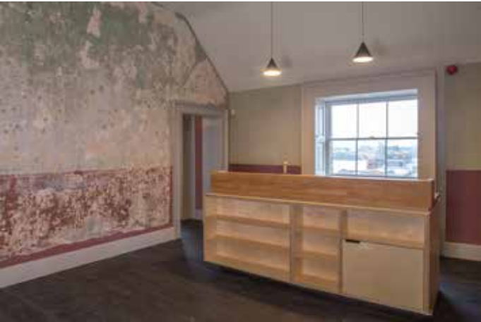
Figure 8. Free-standing kitchen unit in Georgian room. Designed as piece of furniture and carefully located to allow for waste and water pipework to run within floor zone (source: Shaffrey Architects)
