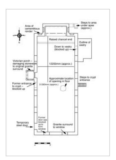
Fig. 7.33 Ground Floor Plan, taken from outline survey carried out on 15 July 2003.
