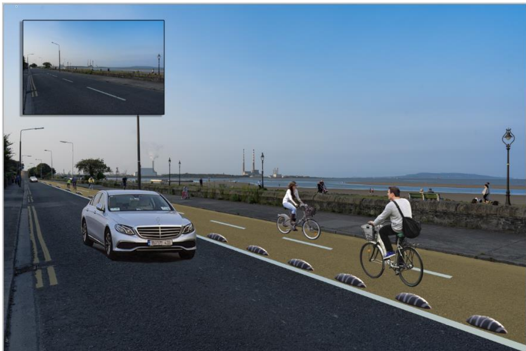
Typical section visualisation showing two way cycling and one way outbound traffic lane
