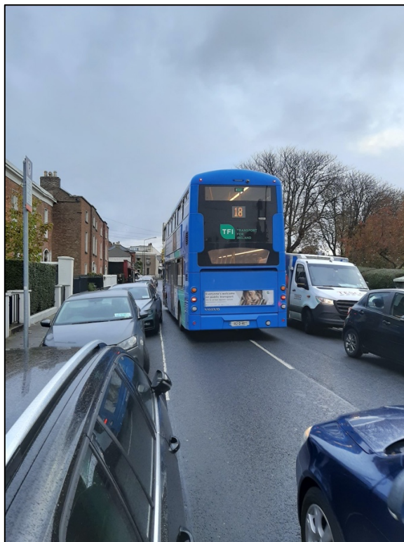
Photo 3. Reason why Number 18 was trying to squeeze pass – because of traffic flowing the opposite direction. Imagine if two opposing buses were attempting to pass one another. Path widths are 2.53m and 1.5m, road width here is 7.45m minus 1.9m (for official parking bay) leaving 5.55m for mobile traffic. – see Fig. 1. above under location (A).
