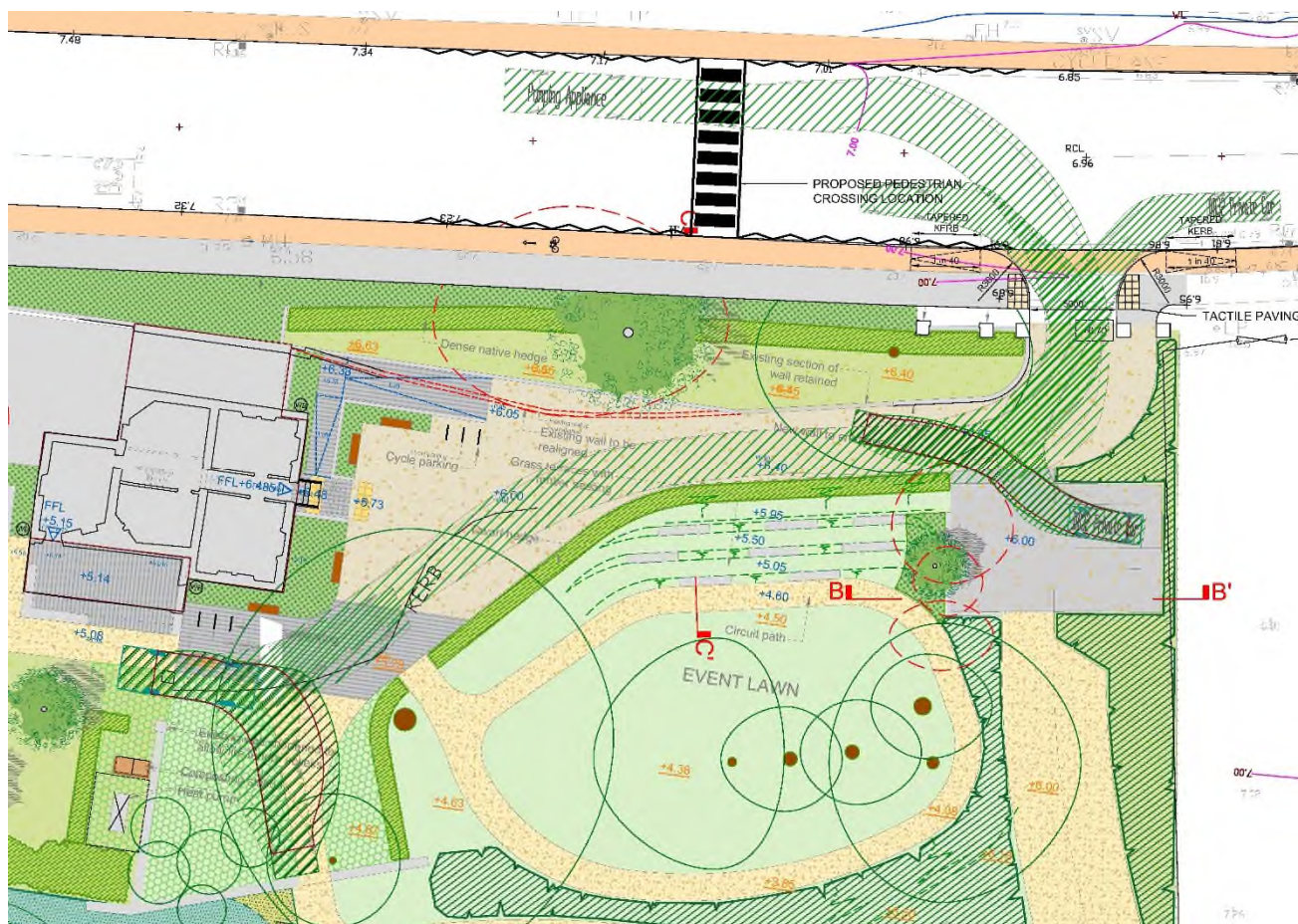
Figure 13 Proposed Entrance – Swept Path Analysis for fire tender and universal access parking and proposed pedestrian crossing.
