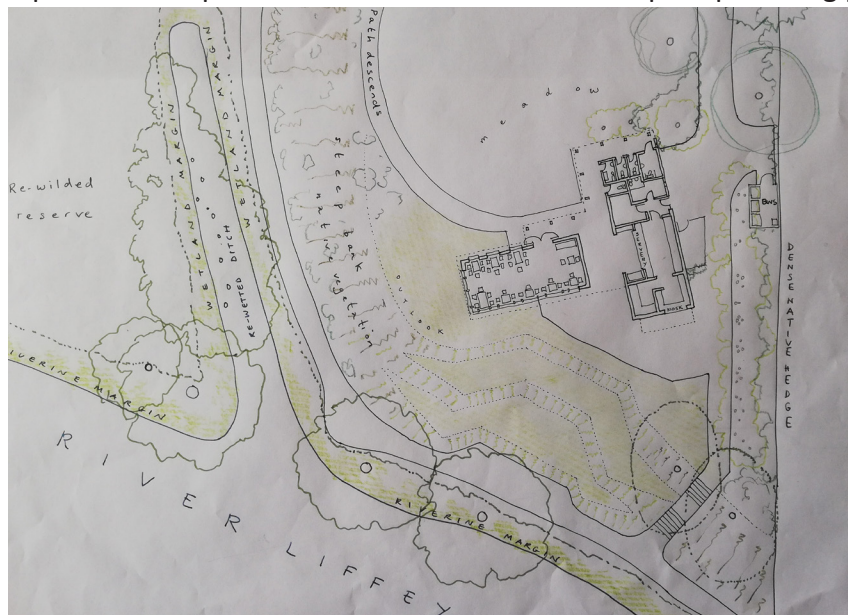
Fig. 5.03 Plan of cafe building, located at the top of the grassy terraces overlooking the river Liffey. Two blocks linked by a covered area. One a generous seating room, the other containing a servery kiosk, kitchen and storage, with public WCs at the north end, located to be accessed from the footpaths. By separating the servery and service building from the internal seating area the concept was that the internal room could also be used for events.
