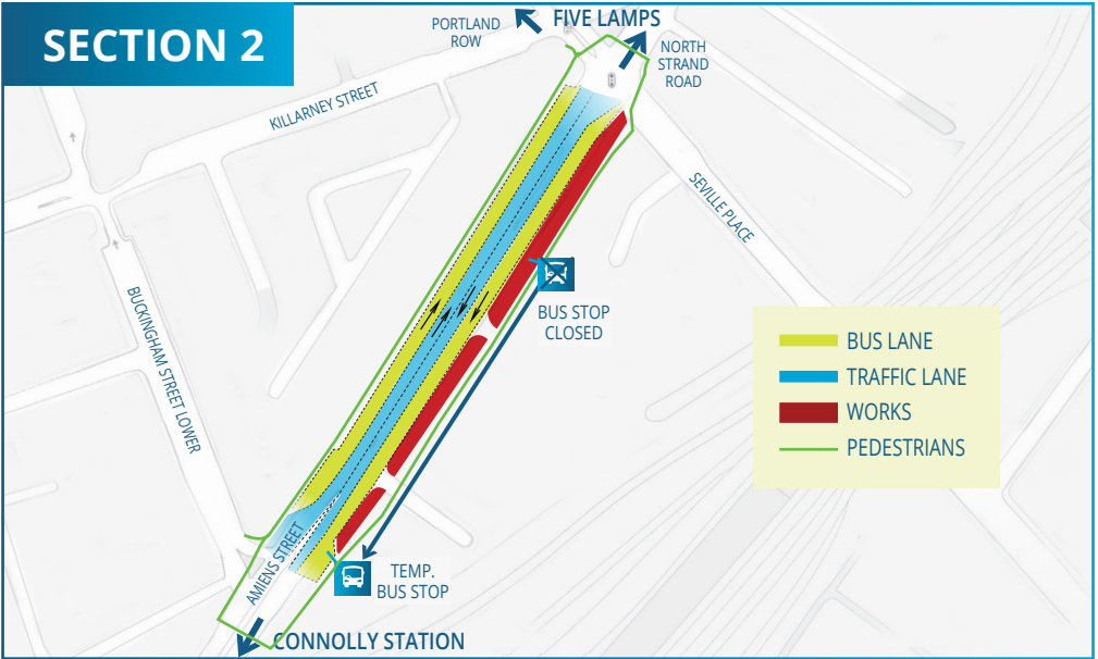
Section 2 Amiens Street - Buckingham Street to the Five Lamps Junction at Portland Row - March to June 2022
