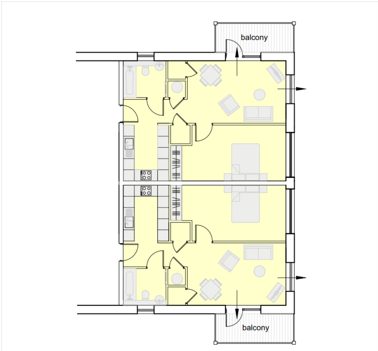
Figure 15.2: Example of Dual Aspect Residential Unit
