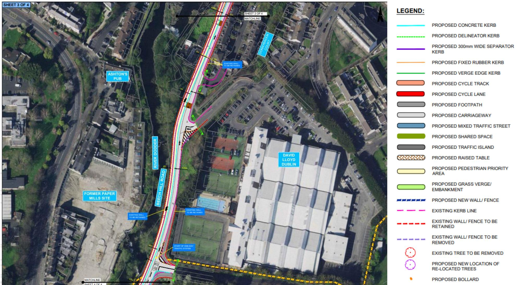
**Figure 4 Donnybrook Rd to Clonskeagh Rd Rapid Deployment Scheme 3/4**
