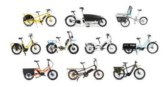
Cargo bikes are bicycles which are designed to carry heavy loads. There are several different designs of cargo bikes, which include tricycle designs. In general they have, either at the front or back of the bike, an additional feature which allows for the transportation of cargo.
