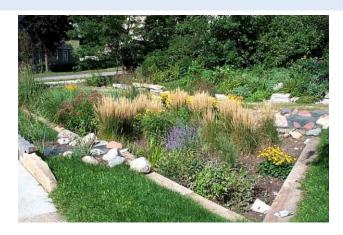
The primary benefit of this strategy is the reduction and prevention of flood damage in an area, as rain gardens can potentially absorb 30% more water than a conventional lawn. It can potentially absorb up to 80% of sediments and 90% of nutrient and pollutants such as oil or heavy metals in runoff from rainfall events too. This strategy also provides advantages associated with greenspace, such as mental health benefits, habitats for animals and carbon sequestration.
