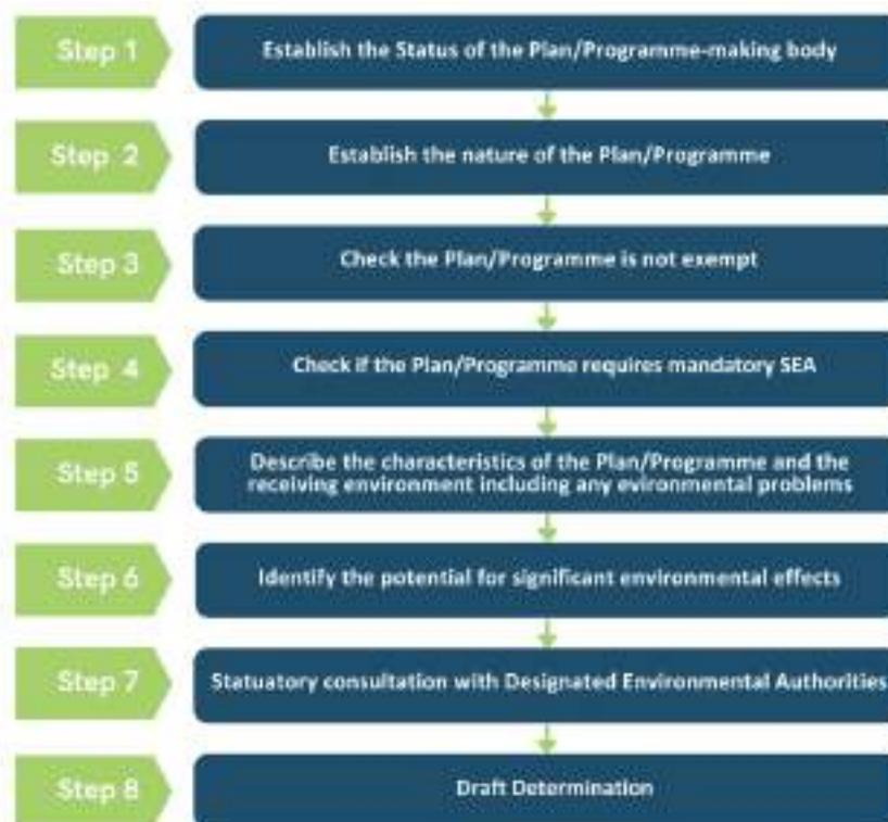
Figure 2-1: SEA Screening steps as per the EPA's Good Practice Guidance on SEA Screening
