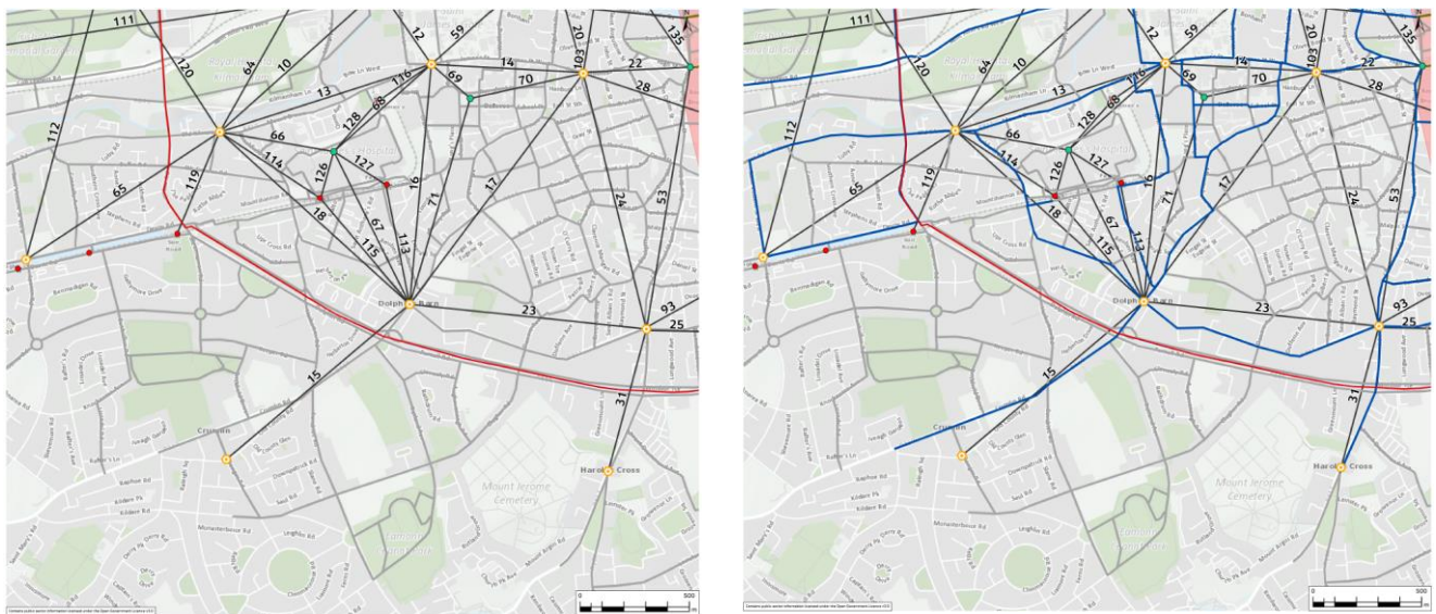
Figure 7-10 Primary route selection in south-west area
