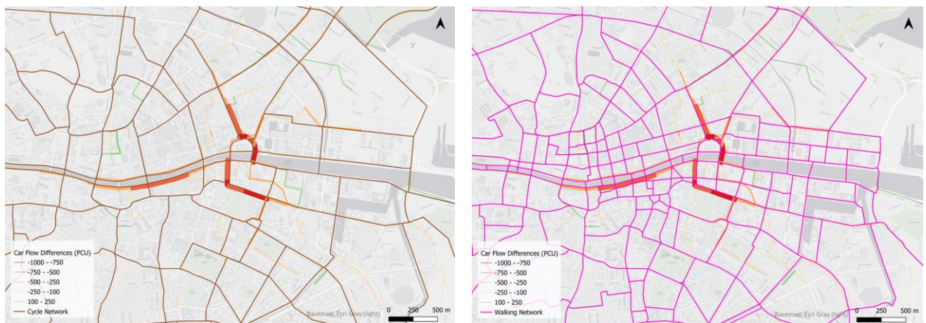
Figure 4-6 Primary Cycling (Left) and Primary Walking (Right) Networks Mapped Over the Difference in Car Flows Between the Do Minimum and Do Something Model Runs (AM peak hour)
