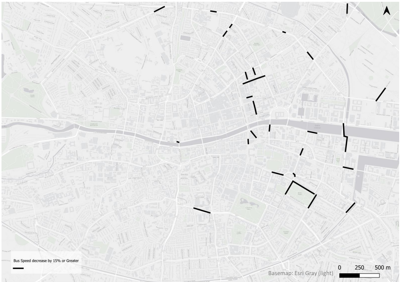
Figure 4-5 Bus-carrying links seeing speed decreases of 15% or more from Do Minimum to Do Something (AM peak hour)
