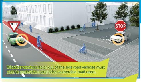
As part of the rollout of the network, continuous footpaths will be provided across minor side roads. The footpath paving is level across the junction establishing the priority of pedestrians and wheelchair users, etc thus improving their safety and convenience.
