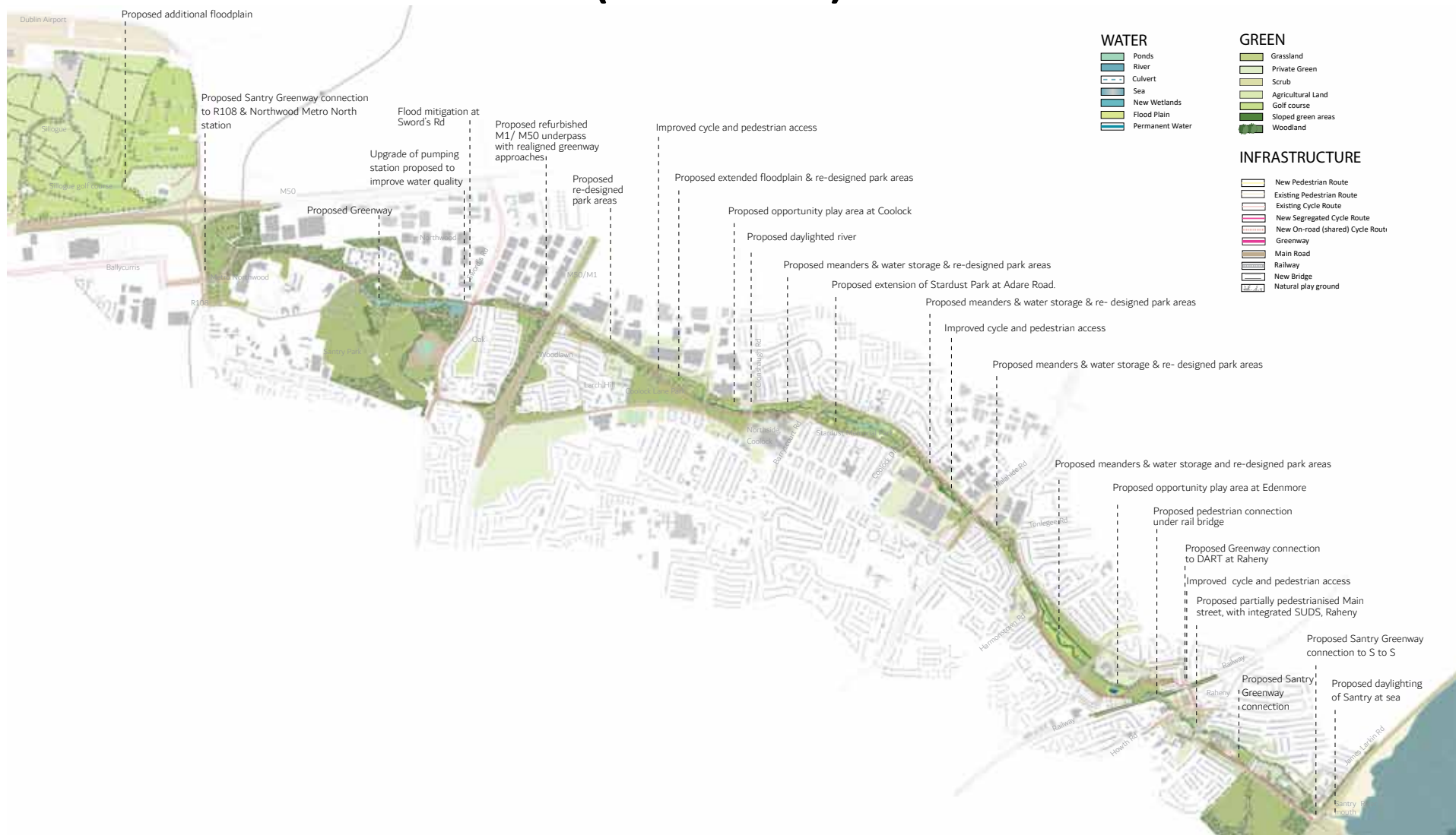
Plan drawing: Masterplan of area showing the proposed situation for flood mitigation, restoration and greenway.
