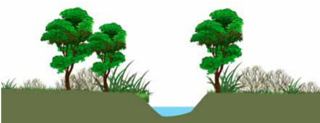
Schematic of riparian zone for the Santry River. Planted riparian buffer should ideally be two bankfull channel widths wide and should remain free from future development.
