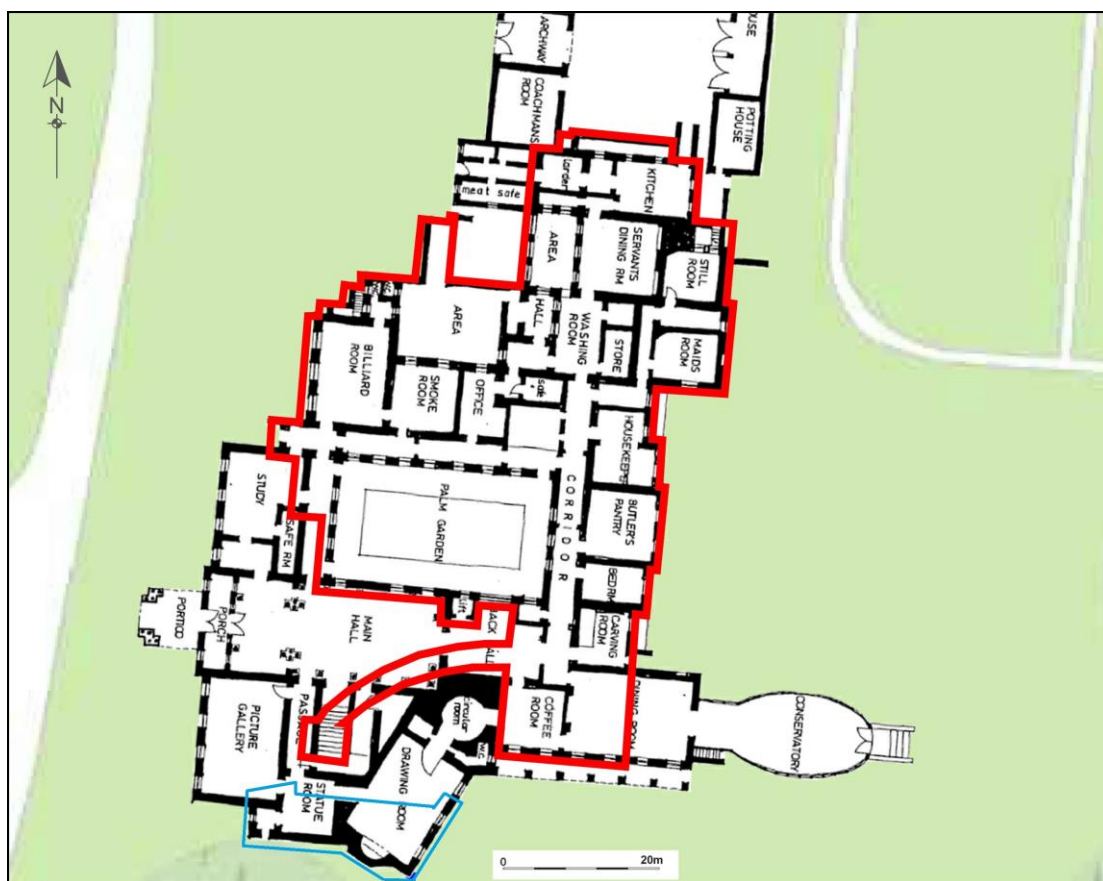
Figure 8 Ground floor plan of St Anne's House with the outline of basement in red, showing location of excavated area in blue (ASI & Sharkey)
