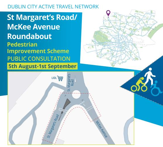
Dublin City Council (DCC), with the support of the National Transport Authority (NTA), propose to enhance pedestrian safety and accessibility at St Margaret's Road/McKee Avenue Roundabout by installing new signalised pedestrian crossings on the southwestern arm (St Margaret's Road) and the southeastern arm (McKee Avenue) of the roundabout. This will Increase safety for pedestrians and vulnerable road users and improve access to the bus stops on McKee Ave and St Margaret's Rd.
