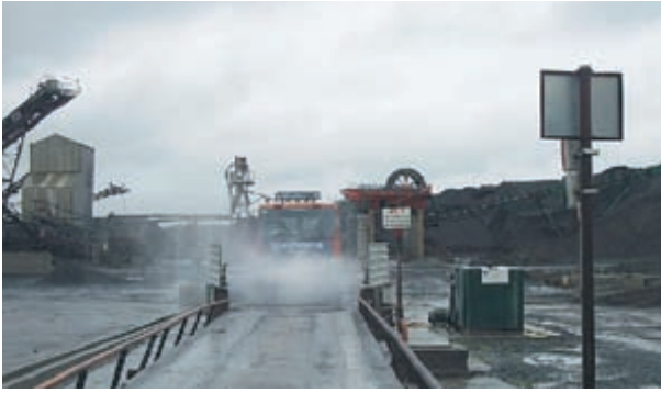
Figure 3.7. Wheelwash facility (Loughnane Concrete, Birr, Co. Offaly).
