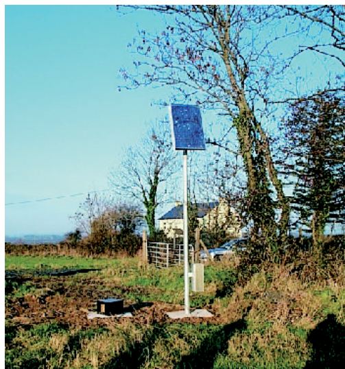
Figure 2.1. Permanent blast monitoring station (Roadstone Provinces Ltd, Brownswood, Co. Wexford).
