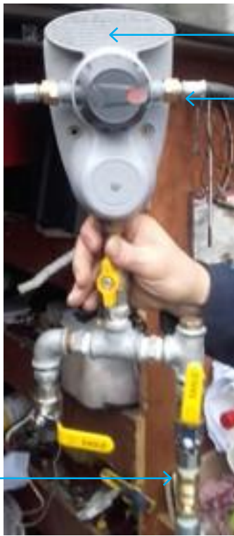
Photograph 9: Low pressure regulator
