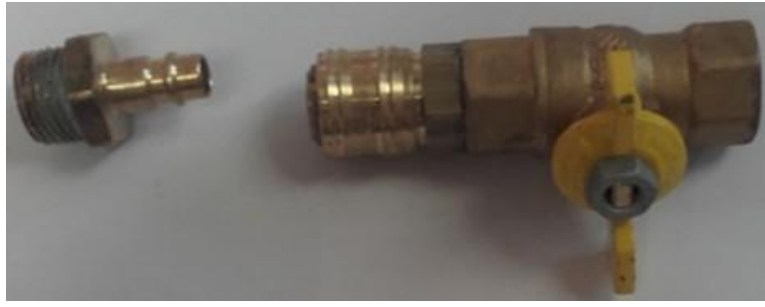
Photograph 4: Bayonet connections all points i.e. plug and play
