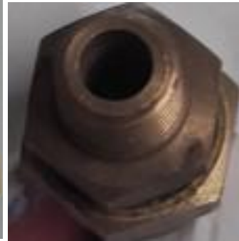
Photograph 7: Non return valves only
