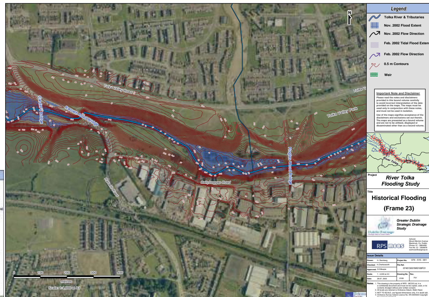
Figure 7 - River Tolka Flooding Study Historical Flooding Map (Frame 23) (this shows roughly the 100 year event)
