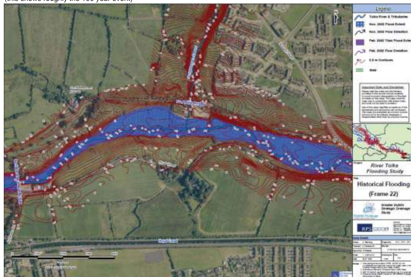
Figure 6 - River Tolka Flooding Study Historical Flooding Map (Frame 22) (this shows roughly the 100 year event)
