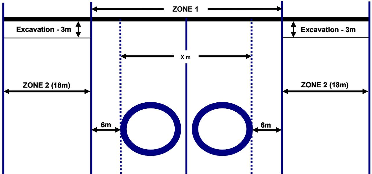
Figure 1: Bored Tunnel – Areas A&B <sup>1</sup>
