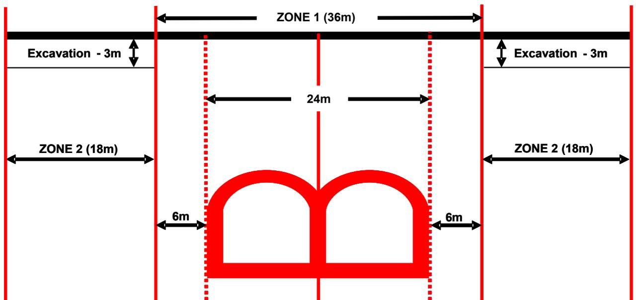
Figure 2: Cut & Cover Tunnel – Area C <sup>1</sup>
